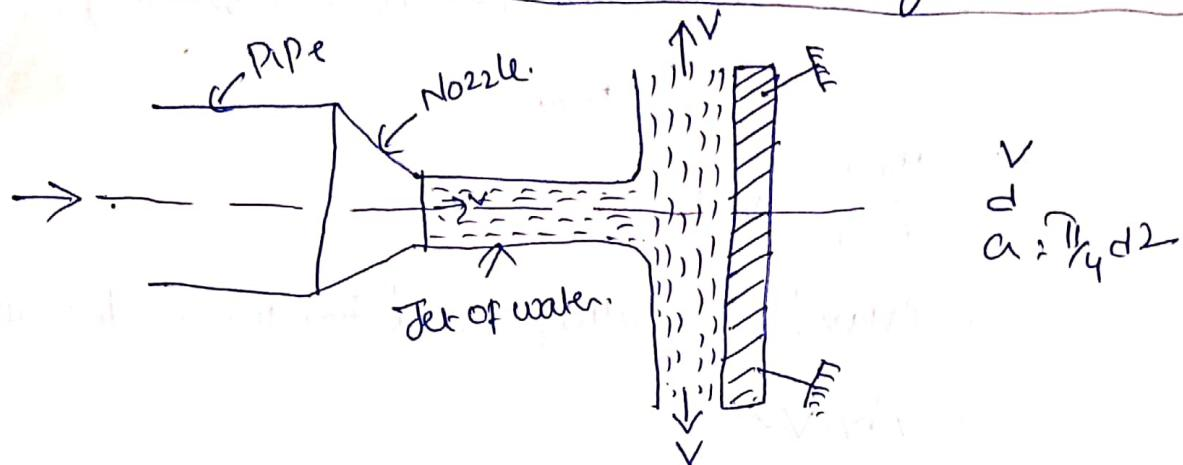
The liquid comes out in the form of a jet from the outlet of a nozzle, which is fitted to a pipe through which liquid is flowing under pressure. If some plate, which may be fixed or moving, is placed in the path of the jet, a force is exerted by the jet on the plate. This force is obtained from Newton's Second law of motion (or) ~~from~~ equation. Thus 'impact of jet' means the force exerted by the jet on a plate which may be stationary (or) moving.
