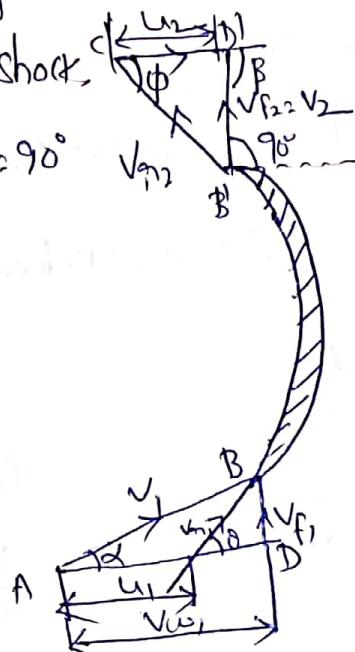
$$\text{where, } V_{f_1} = V_i \sin \alpha = 40 \times \sin 30 = 20 \text{ m/sec}$$
