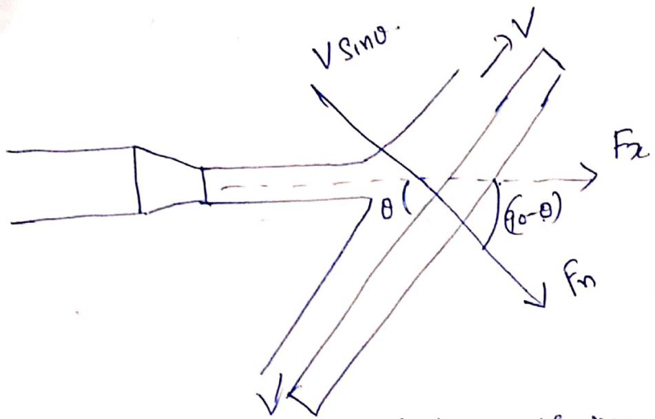
$F_n = m a v (v \sin \theta)$  or  $\text{jet before striking in the normal direction}$
