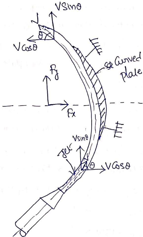
Let the jet strikes the curved plate at one end tangentially as shown in fig. Let the curved plate is symmetrical about x-axis. Then the angle made by the tangents at the two ends of the plate will be same.
