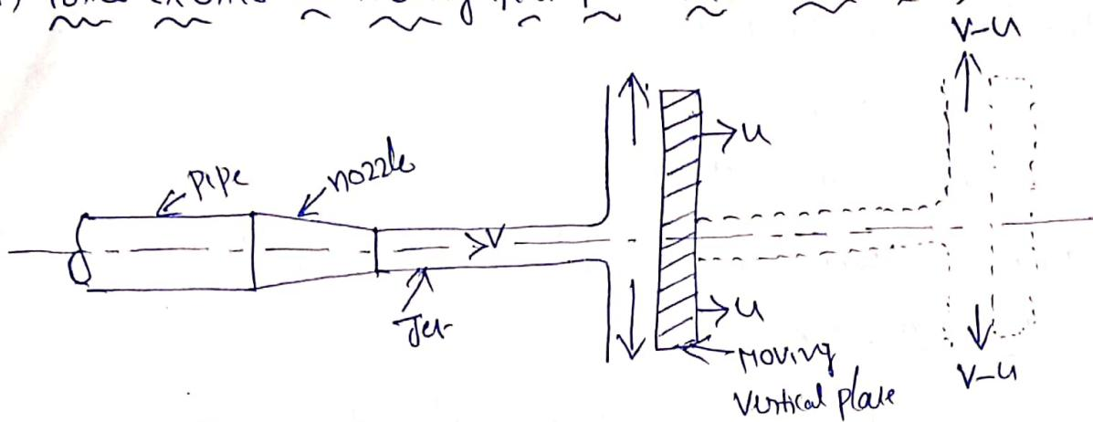
The above figure shows a fluid jet striking a flat vertical plate moving with a uniform velocity away from the jet.
