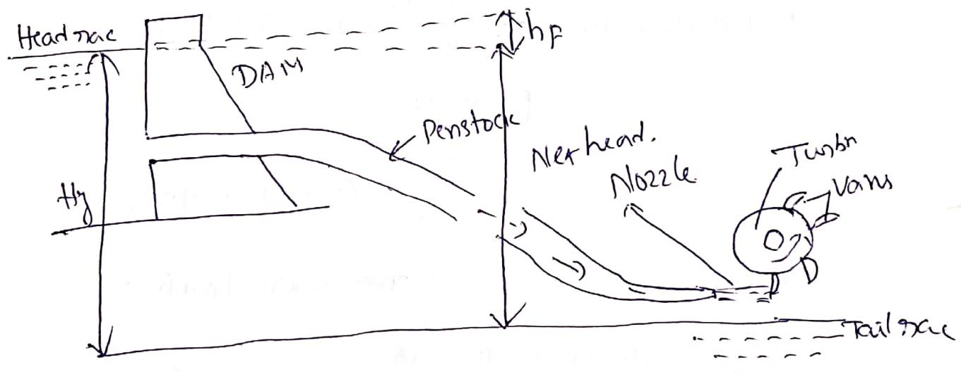
① Gross head: The difference between The head race level and tail race level when no water is flowing is known as Gross head.  $H_g$
