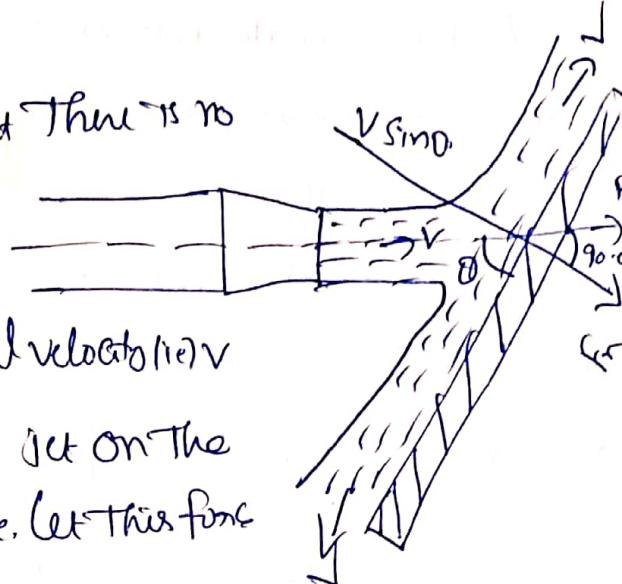
$$\therefore F_n = \max [I.v \text{ in } n \text{ direction} - F_r \text{ in } n \text{ direction}]$$
