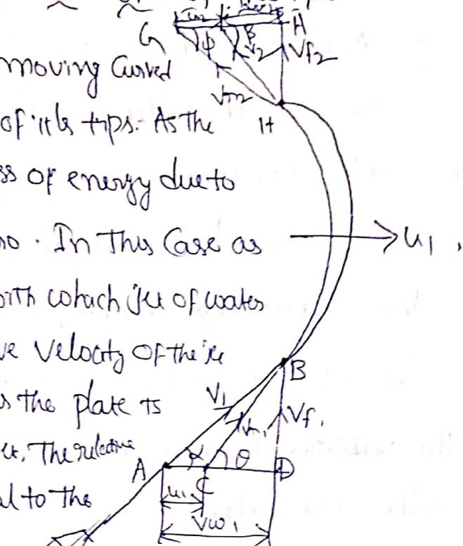
Let  $V_1$  : Velocity of the jet at inlet
