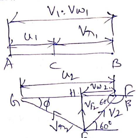
$$V_{w2} \cdot U_2 - V_{h2} \cos \phi = 5 \text{ m/s.}$$
